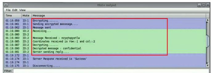
Fig. 8. Encryption Decryption Process.
