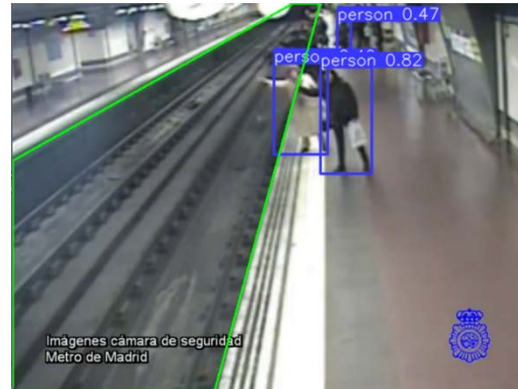
Fig. 4. BBox generated by object detection system.
